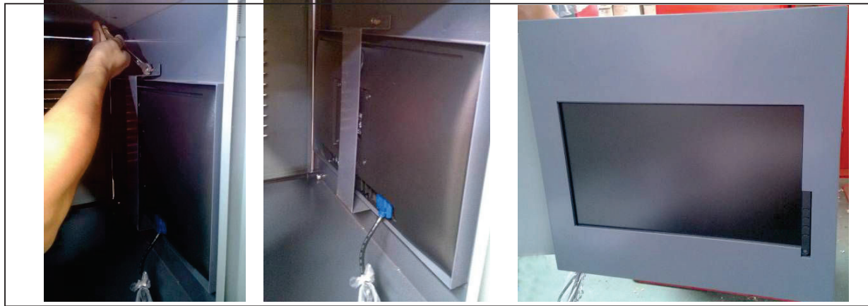
Fig. 2-35 Installation of Display
