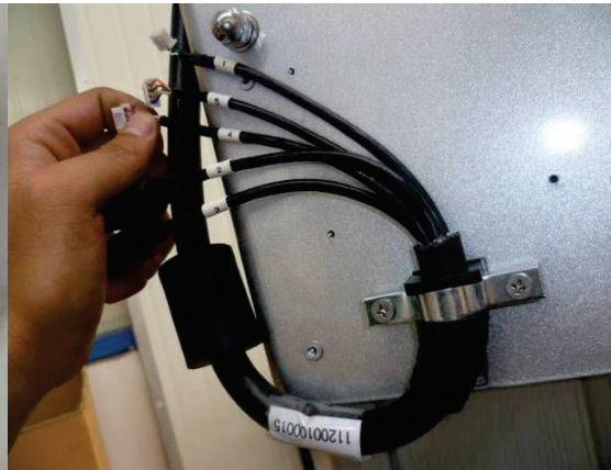
(Fig.2-12 Circuit Connection 1- Internal Circuit Diagram of Control Panel) (Fig. 2-13 Circuit Connection 1- Connection Plug of Control Panel)
