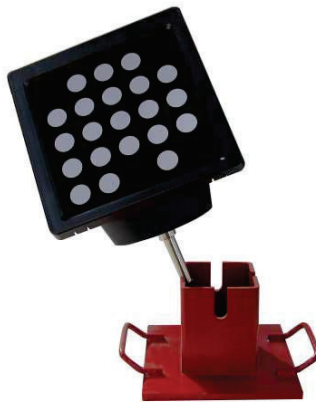
Fig. 2-48 Target Board Used for Measuring the Vehicle Height
